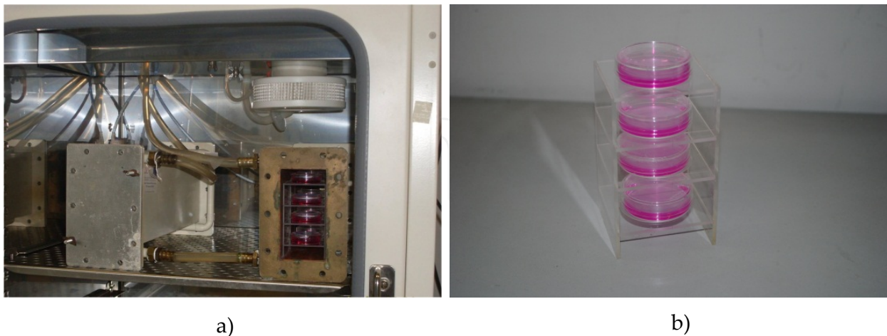
Figure 5. Short-circuited waveguides hosted in a cell culture incubator (panel a) and sample holder hosting cell cultures to be placed in the waveguide (panel b)
