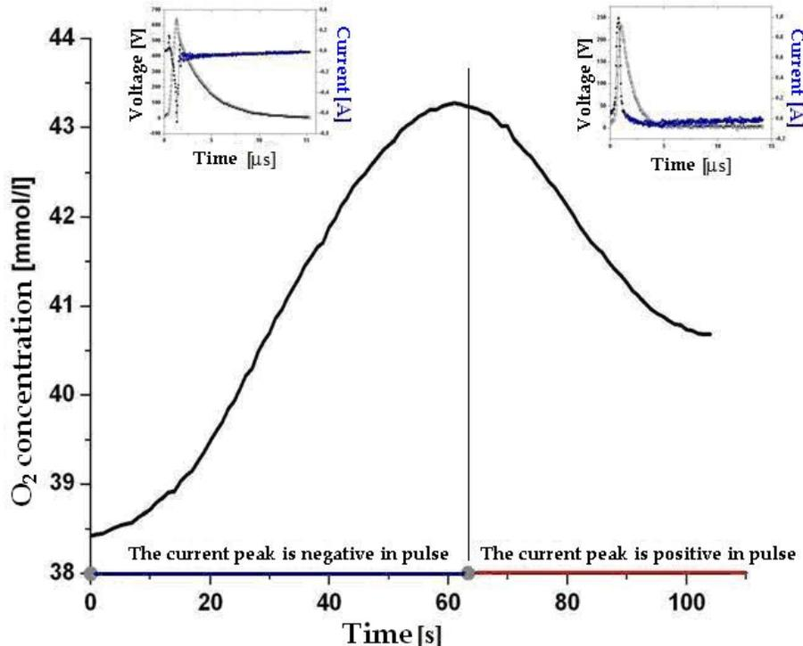
**Figure 15.** Dissolved oxygen concentration near the cathode in two regimes of pulse generator – when current peak is negative (left, dissolved oxygen concentration is increasing) and positive (right, dissolved oxygen concentration is decreasing).
