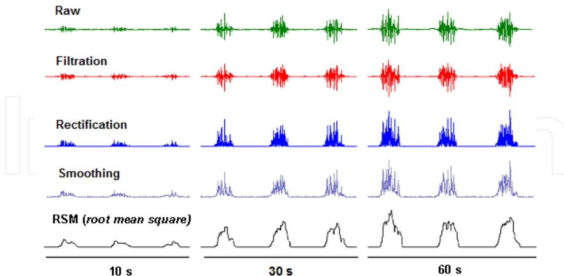
**Figure 2.** EMG signal process recommended. Green: The raw signal, no treatment was applied until this moment; Red: Filtrated signal, a limit was created for the signal, excluding everything out of it; Blue: Rectified signal, all negative values were transformed in positive ones and added; Purple: the smoothed signal, a linear enveloped was created and the extreme parts of the signal was excluded; Black: The RMS values after all the treatments.
