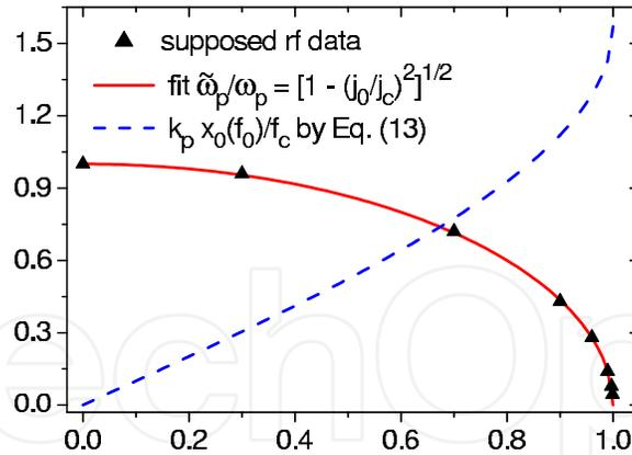
**Figure 5.** The pinning potential reconstruction procedure: step 1. A set of  $[(\tilde{\omega}_p/\omega_p)_i, (j_0/j_c)_i]$  points ( $\blacktriangle$ ) has been deduced from the supposed measured data and fitted as  $\tilde{\omega}_p/\omega_p = \sqrt{1 - (j_0/j_c)^2}$  (solid line). Then by Eq. (17)  $x_0(f_0) = (f_c/k_p) \arcsin(f_0/f_c)$  (dashed line).
