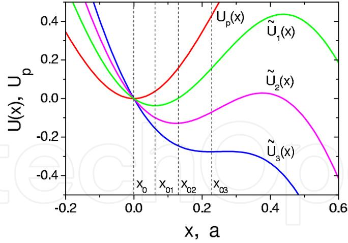
**Figure 4.** Modification of the effective pinning potential  $\tilde{U}_i(x) \equiv U_p(x) - f_{0i}x$ , where  $U_p(x) = (U_p/2)(1 - \cos kx)$  is the WPP, with the gradual increase of  $f_0$  such as  $0 = f_0 < f_{01} < f_{02} \lesssim f_{03} = f_c$ , i.e., a vortex is oscillating in the gradually tilting pinning potential well in the vicinity of the rest coordinate  $x_{0i}$ .
