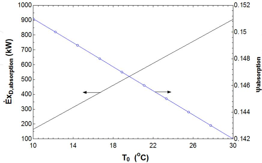
**Figure 5.** Exergy destruction rate and exergy efficiency of the absorption cooling and heating system depending on ambient temperature changes
