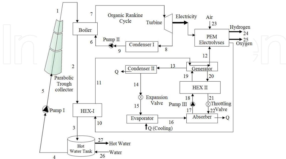
Figure 1. The Solar multi-generation energy production system
