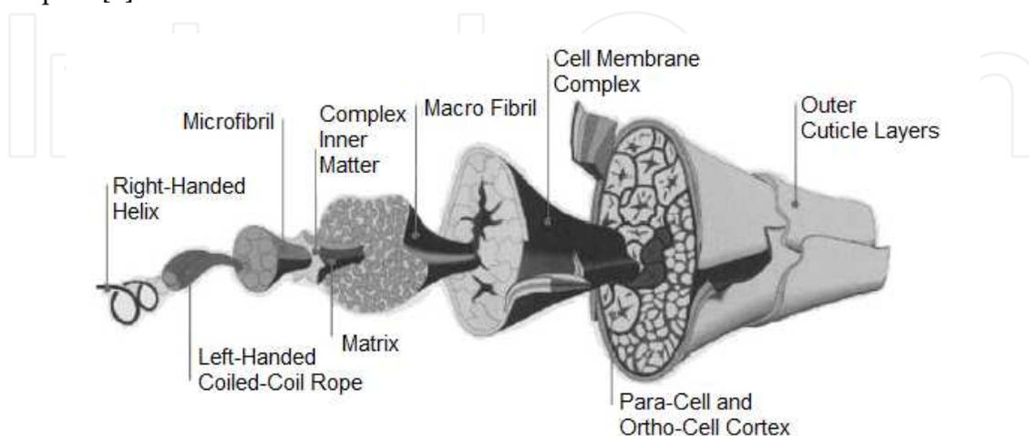
**Figure 1.** Cross-section diagram of a merino wool fiber [6]
