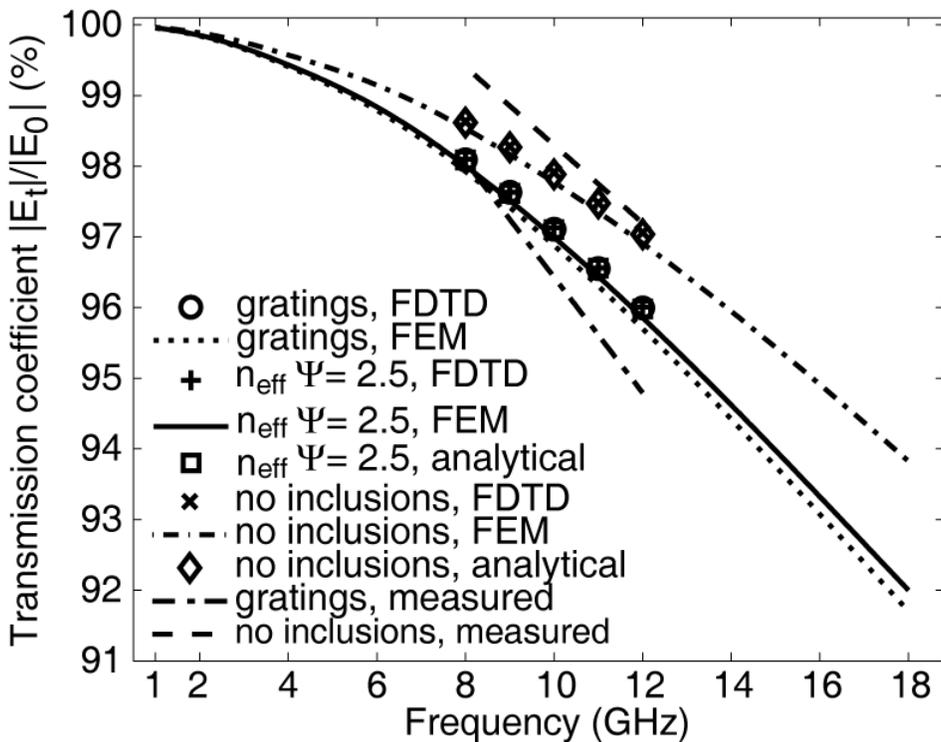
**Figure 7.** Plot of the transmission coefficient for a grating structure. The experimental data follows the same trend as the numerical FDTD and FEM calculations obtained for grating, homogenised and reference structure. Grating parameters:  $f = 0.3$ ,  $\Lambda = 500 \mu\text{m}$ ,  $AR = 1$ ; substrate: thickness  $762 \mu\text{m}$ ,  $\epsilon_r = 3.66$ .
