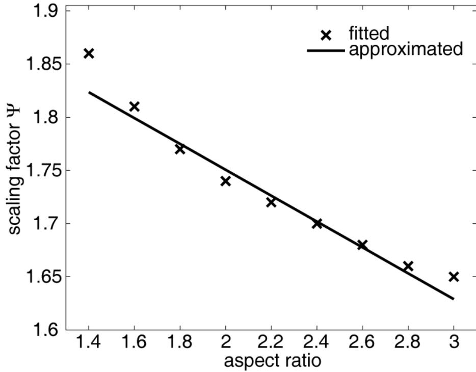
**Figure 2.** Plot of the scaling factor  $\Psi$  obtained for an example grating structure. The fitted values (crosses) show good agreement with approximated data (lines). Grating parameters:  $f = 0.5$ ,  $\Lambda = 100 \mu\text{m}$ ,  $\nu = 5 \text{ GHz}$ ,  $\epsilon = 6.25$ ,  $1.4 \leq x_{AR} \leq 3$ .
