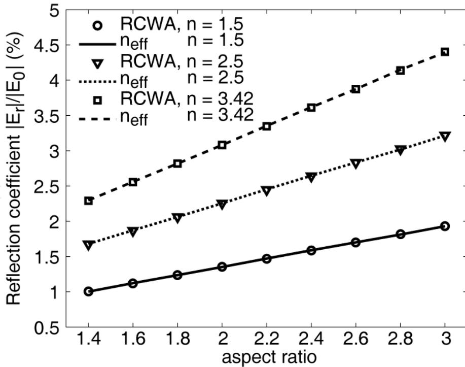
**Figure 3.** Plot of the reflection coefficient obtained from a subset of the gratings studied, as a function of aspect ratio and host permittivity. Results from the homogenised model are drawn as lines, while those from the detailed structure simulated with RCWA are plotted as markers. Fixed parameters:  $\nu = 5 \text{ GHz}$ ,  $f = 0.5$ .
