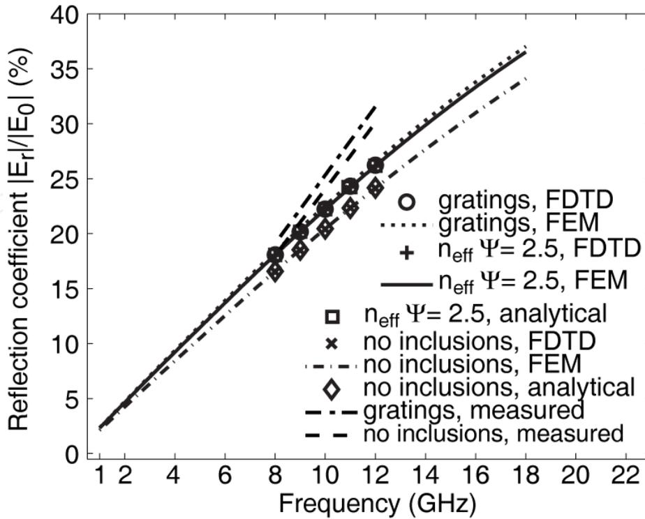
**Figure 6.** Plot of the reflection coefficient for a grating structure. The experimental data follows the same trend as the numerical FDTD and FEM calculations obtained for grating, homogenised and reference structure. Grating parameters:  $f = 0.3$ ,  $\Lambda = 500 \mu\text{m}$ ,  $AR = 1$ ; substrate: thickness  $762 \mu\text{m}$ ,  $\epsilon_r = 3.66$ .
