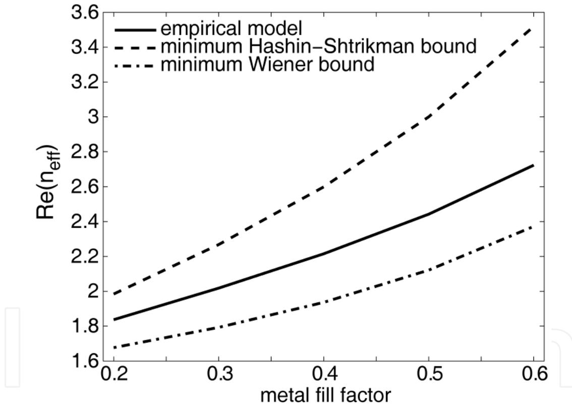
**Figure 4.** Plot of the real part of the effective refractive index of the grating structure compared with theoretical bounds. Grating parameters:  $x_{AR} = 1$ ,  $\epsilon = 11.7$ ,  $\Lambda = 100\mu\text{m}$ ,  $\nu = 5\text{GHz}$ ,  $0.2 \leq f \leq 0.6$ .
