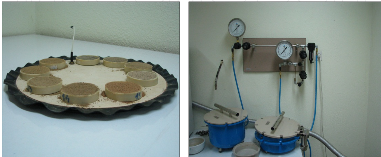
Figure 2. Preparing soil and placing samples on Bar extractor and Porous plate extractor
