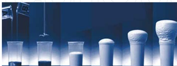
Figure 2. Polymerization of the palm-based polyurethane
