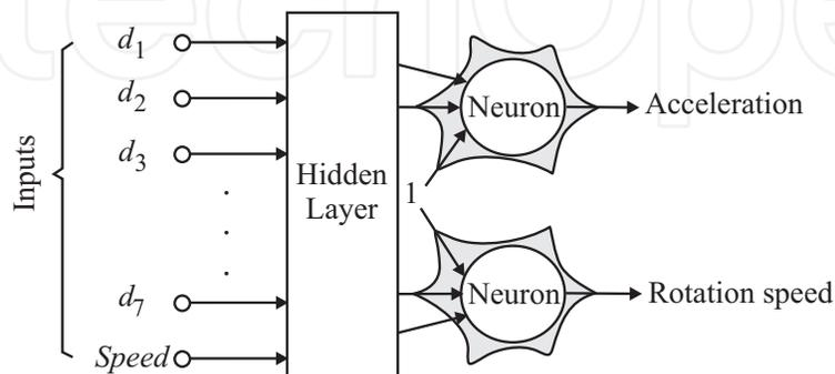
Figure 12. Artificial Neural Network for driving the car.
