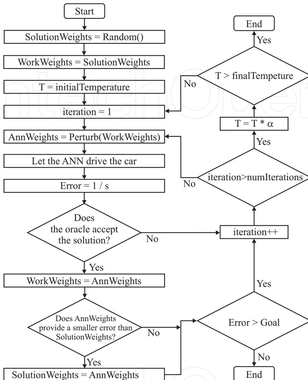
Figure 13. Flow diagram for simulated annealing evolution.
