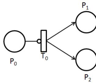
Figure 5. PN with an inhibitor arc.
