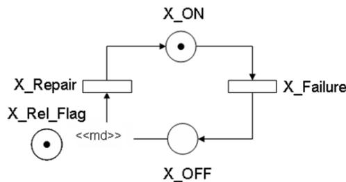
**Figure 17.** Simple component model
