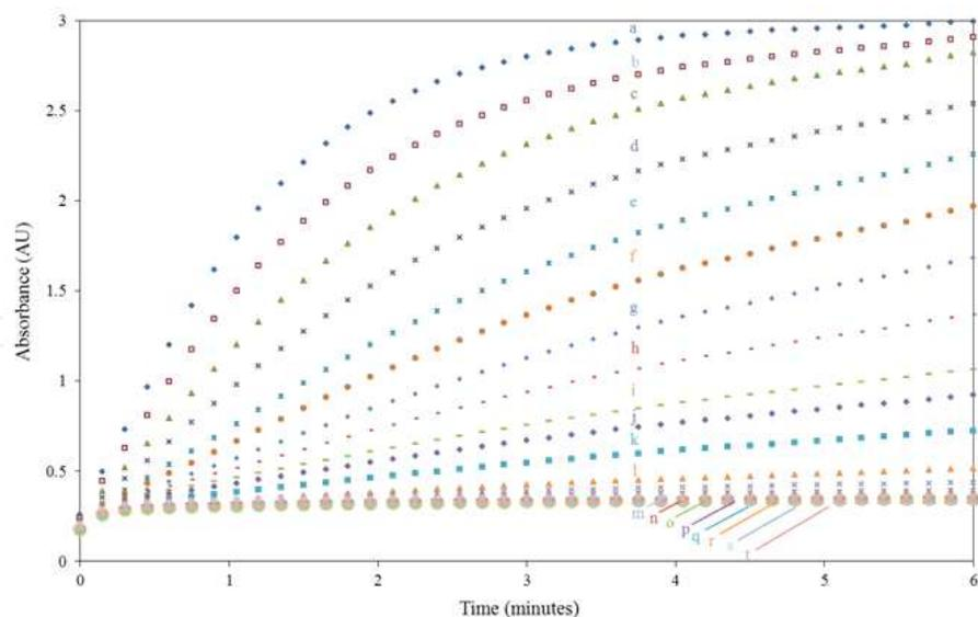
**Figure 7.** Monitoring of reaction curves of *t*-TBH in the concentrations from 0.06 to 1000  $\mu\text{M}$  - a) 1000, b) 750, c) 500, d) 375, e) 250, f) 187, g) 125, h) 94, i) 63, j) 47., k) 31, l) 15.6, m) 7.8, n) 3.9, o) 1.9, p) 0.9, q) 0.4, r) 0.2, s) 0.1, and t) 0.06  $\mu\text{M}$  in the time interval from 0 to 6 minutes. All analyses were carried out in triplicates.
