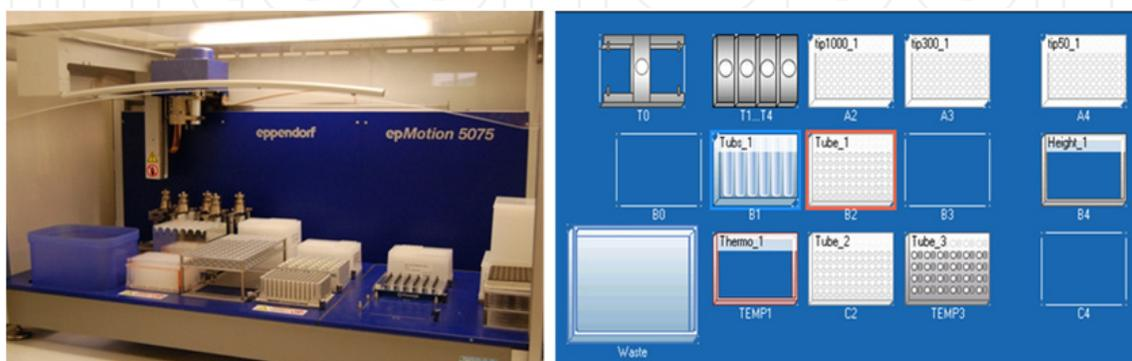
**Figure 4.** epMotion 5075 automated pipetting system from frontal part.
