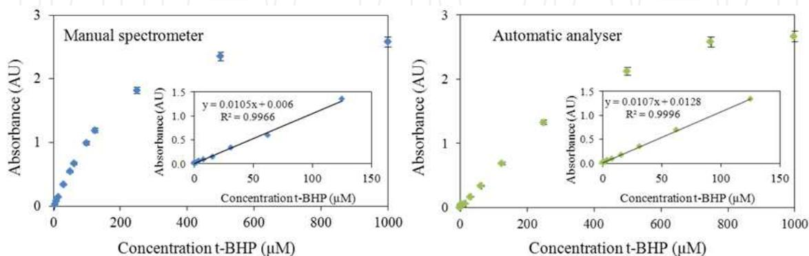
**Figure 8.** Dependence of absorbance on applied *t*-BHP concentration measured by manual spectrophotometer SPECOL 210 and automated analyser BS-400. All analyses were carried out in triplicates. For other experimental detail, see Fig. 7.
