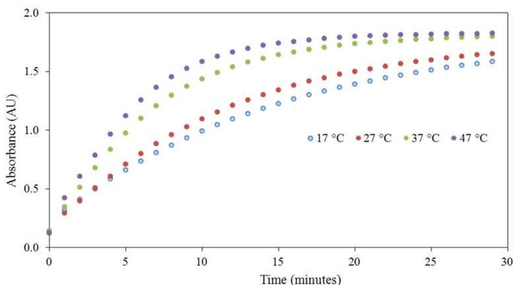
**Figure 6.** Dependences of representative concentration (62.5  $\mu\text{M}$ ) of applied *t*-BHP on temperature conditions (17, 27, 37 and 47  $^{\circ}\text{C}$ ) and the time of interaction. Detected at 591 nm, interval of record is 1 minute, interval period 0 - 30 minutes. All analyses were carried out in triplicates.
