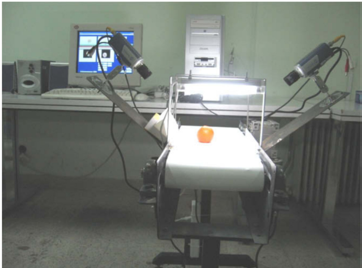
Figure 8. The developed machine vision system.
