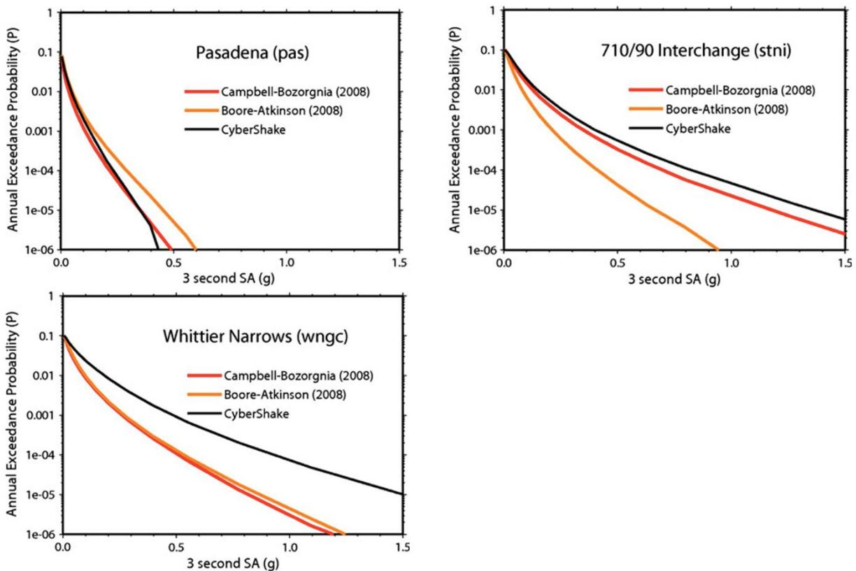
**Figure 2.** Hazard curves derived from three different methods at three sites, PAS, STNI and WNGC, in Los Angeles region. The red lines represent the results of using Campbell and Bozorgnia's [8] method; the orange lines represent the results of Boore and Atkinson's [20] method; the black lines represent the results of CyberShake. Adopted from [5].
