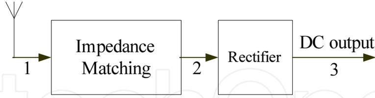
**Figure 3.** RF to DC radio-triggered wake-up circuit
