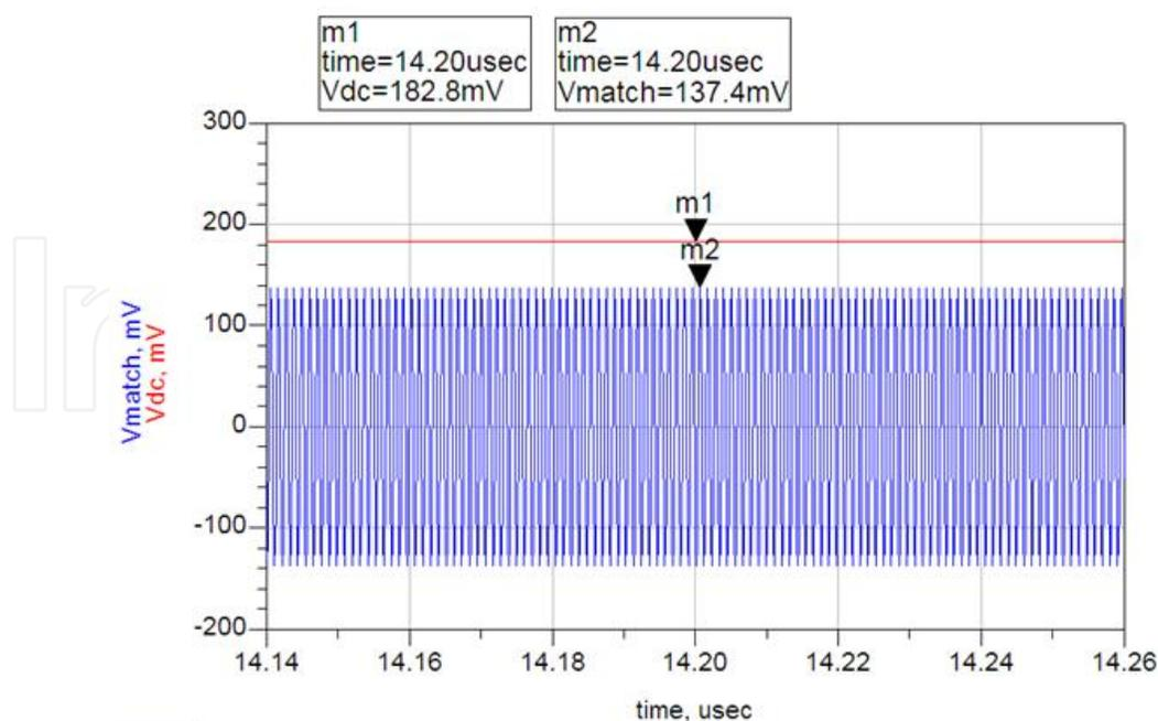
**Figure 9.** Voltage of L type matching network with input signal of 1.7uW (-27.7dBm)
