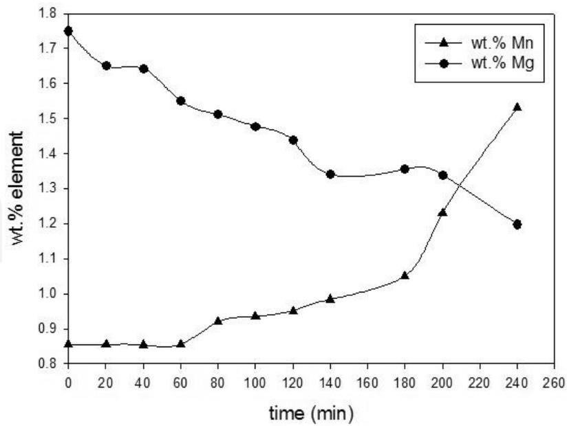
**Figure 8.** Variation of the concentrations of Mn and Mg, with respect to treatment time, during the metallothermic reduction of  $Mn_2O_3$ , for a target Mn concentration of 1.50 wt. % at constant temperature.
