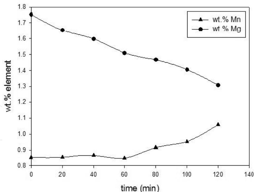
**Figure 5.** Variation of the concentrations of Mn and Mg, with respect to treatment time, during the metallothermic reduction of  $Mn_2O_3$ , for a target Mn concentration of 1 wt. % at constant temperature.
