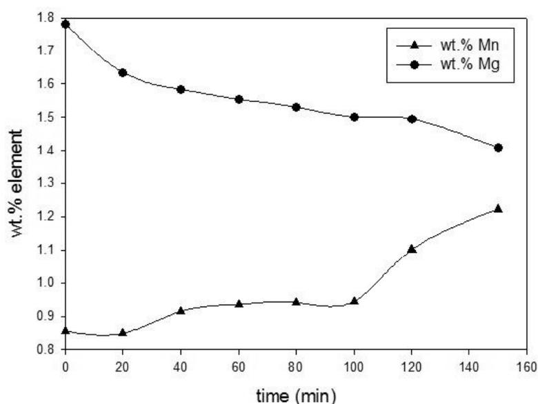
**Figure 7.** Variation of the concentrations of Mn and Mg, with respect to treatment time, during the metallothermic reduction of  $Mn_2O_3$ , for a target Mn concentration of 1.25 wt. % at constant temperature.
