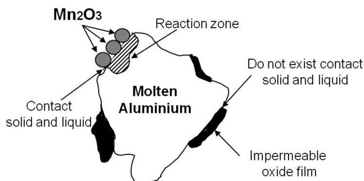
**Figure 1.** Scheme of the aluminothermic reduction of  $Mn_2O_3$  [10,11].
