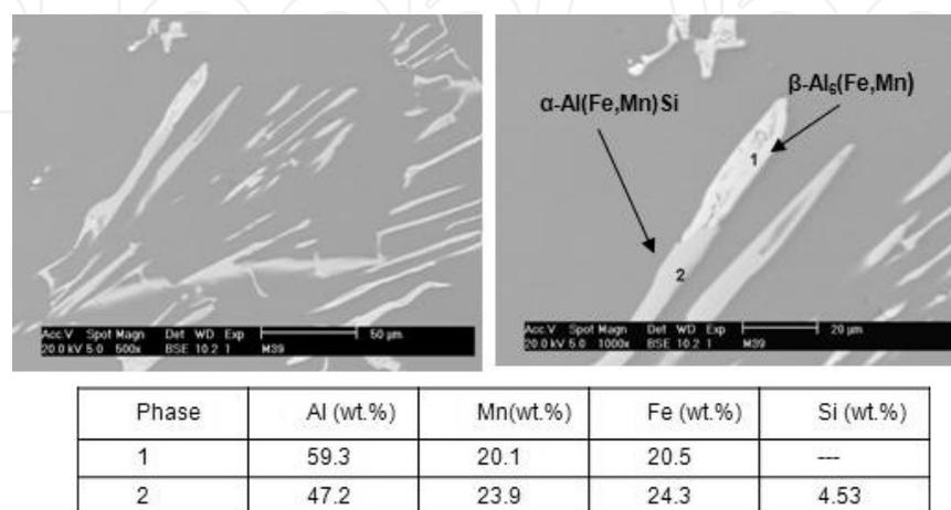
**Figure 15.** SEM micrograph of an Al-1 wt. %Mn alloy showing the morphology of the  $\beta-Al_6(Fe,Mn)$  and  $\alpha-Al_{12}(Fe,Mn)_3Si$  phases particles after a homogenizing treatment at  $550^\circ C$  for 15 hours.
