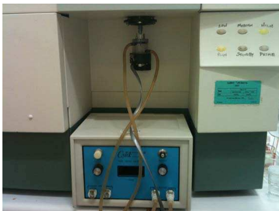
Fig. 1. A picture of Time Zero module integrated with a FACSCalibur flow cytometer
