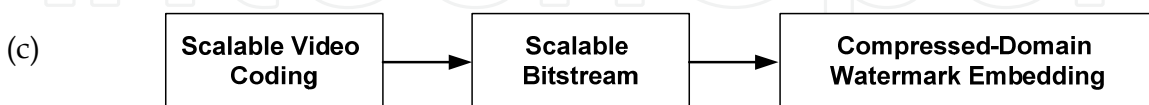
Fig. 3. Three different watermarking embedding schemes by using spatial Scalable Video Coding (Meerwald, P. & Uhl, A., 2010a): a) Watermark embedding prior to the video encoding; b) Integrated watermark embedding and coding; and c) Compressed-domain embedding after encoding.
