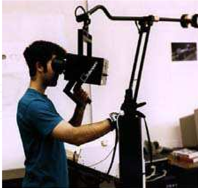
Fig. 2. A binocular omniorientation monitor (BOOM)
