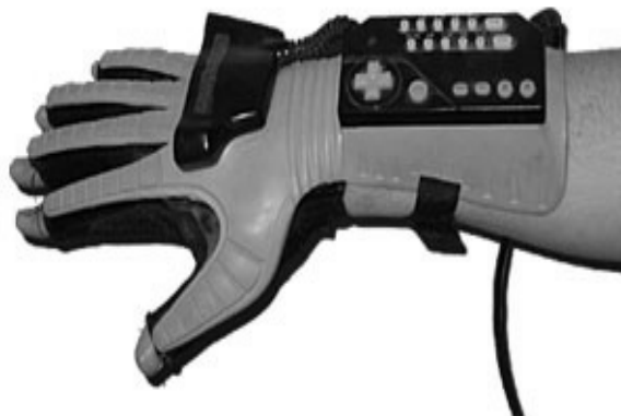
Fig. 5. An instrumented glove (Nintendo power glove)
