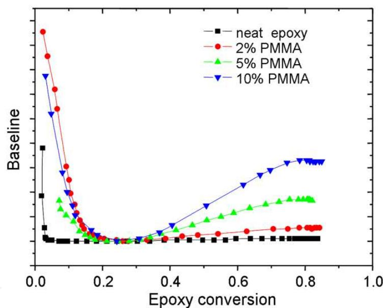
Fig. 12. Baseline from FTIR spectra at  $6300\text{ cm}^{-1}$  as a function of epoxy conversion of DGEBA/PAMS for different weight concentrations of PMMA as modifier (Adapted with permission from (Cabanelas, J.C.; Serrano, B.; Baselga, J. *Macromolecules*, Vol.38, No.3, (2005)). Copyright (2005) American Chemical Society).
