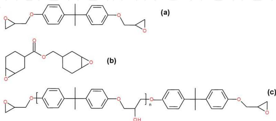
Fig. 2. Chemical structures of common epoxy resins: a) 2,2-Bis[4-(glycidyloxy)phenyl]propane (DGEBA); b) 3,4-Epoxy cyclohexylmethyl-3,4-epoxy cyclohexane carboxylate (ECC); c) DGEBA oligomer,  $n = 0.2$  typically.
