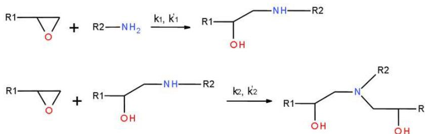
Fig. 3. Epoxy-amine reaction scheme.  $k_1$  and  $k_2$  correspond to the non catalyzed kinetic constants for the addition of primary and secondary amines respectively.  $k'_1$  and  $k'_2$  correspond to the catalyzed processes.
