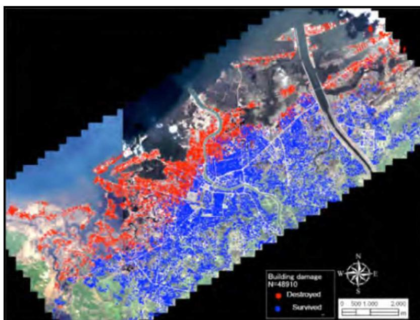
Fig. 4. Detection of tsunami damaged buildings (Red dots indicate damaged buildings and blue dots indicate undamaged buildings) from IKONOS imageries (Source: Suppasri et al., 2012)
