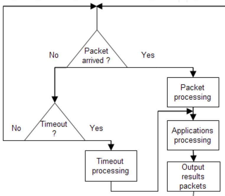
Fig. 7. The main control loop for LWIP stack
