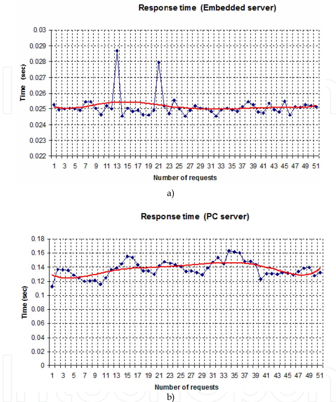
Fig. 17. The response time: a) Embedded server; b) PC server (red line is a trend line)
