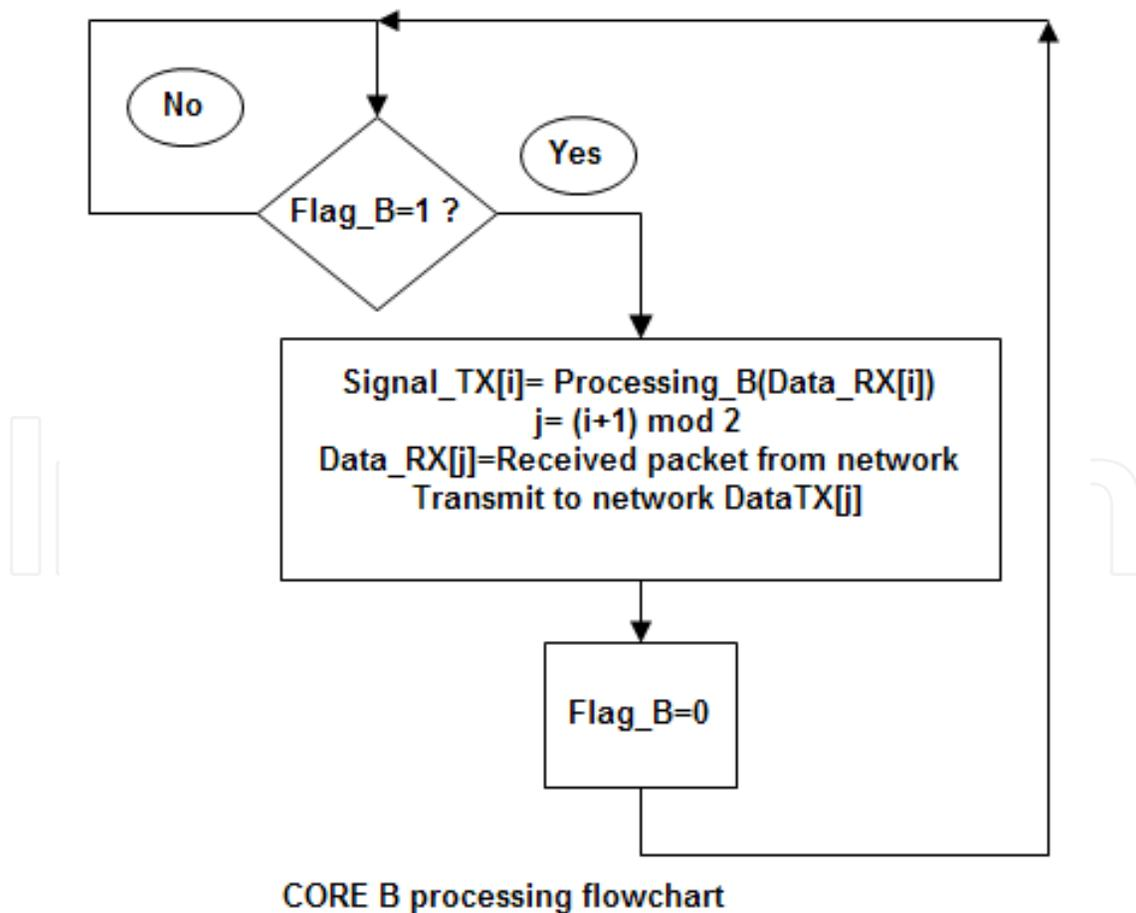
Fig. 11. Program flowchart in core B
