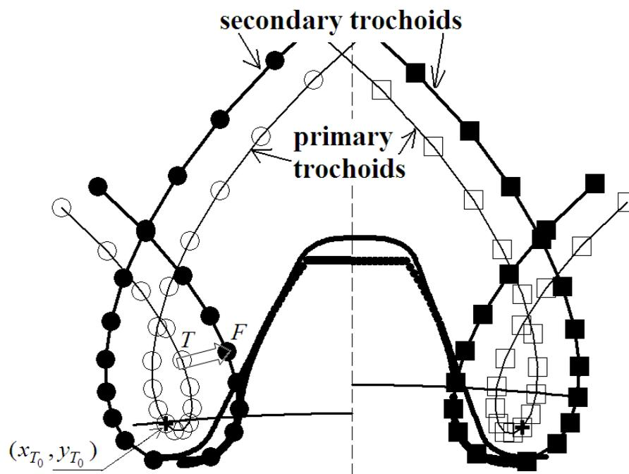
Fig. 6. Trochoidal paths of the rack-type cutter tip
