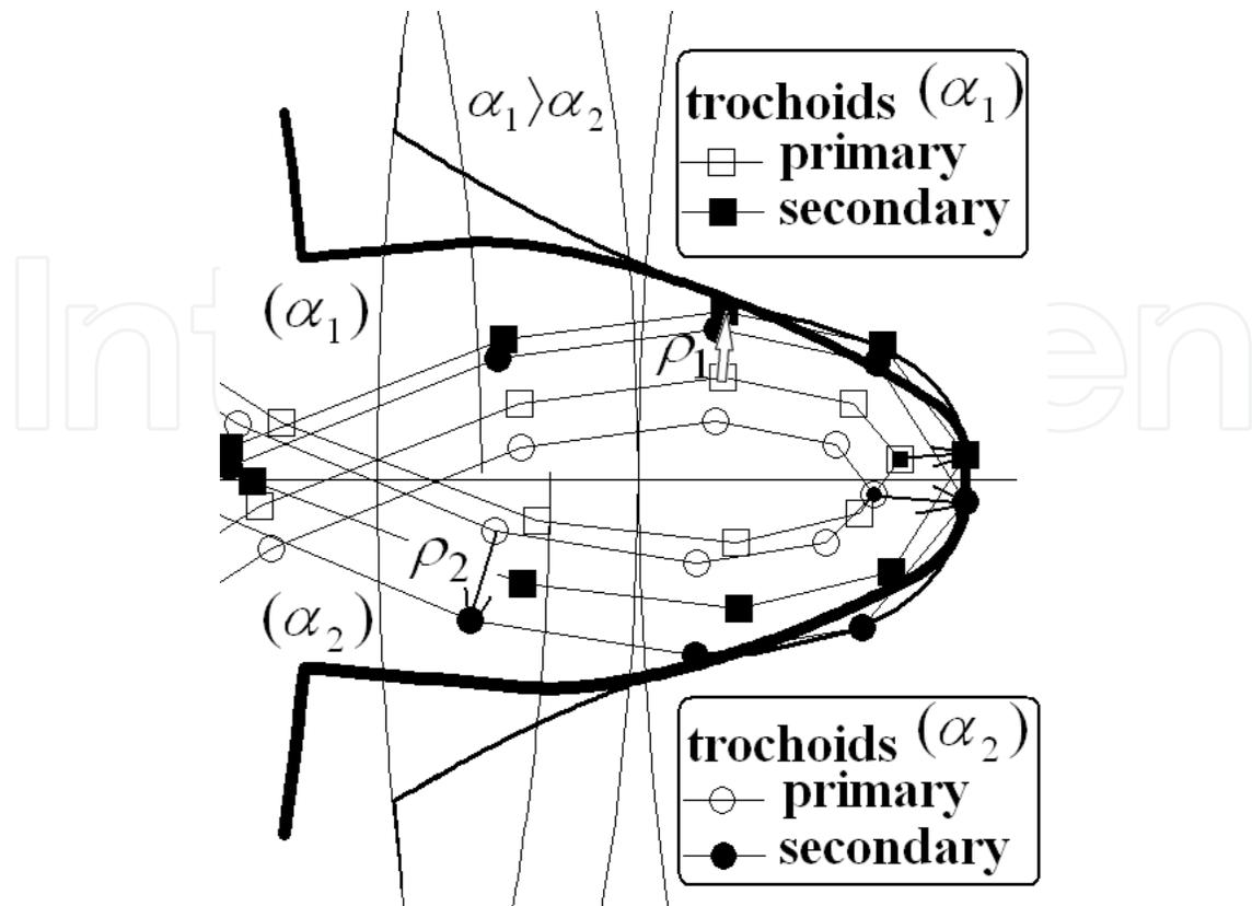
Fig. 12. Cutter with a smaller rounding radius for higher pressure angle
