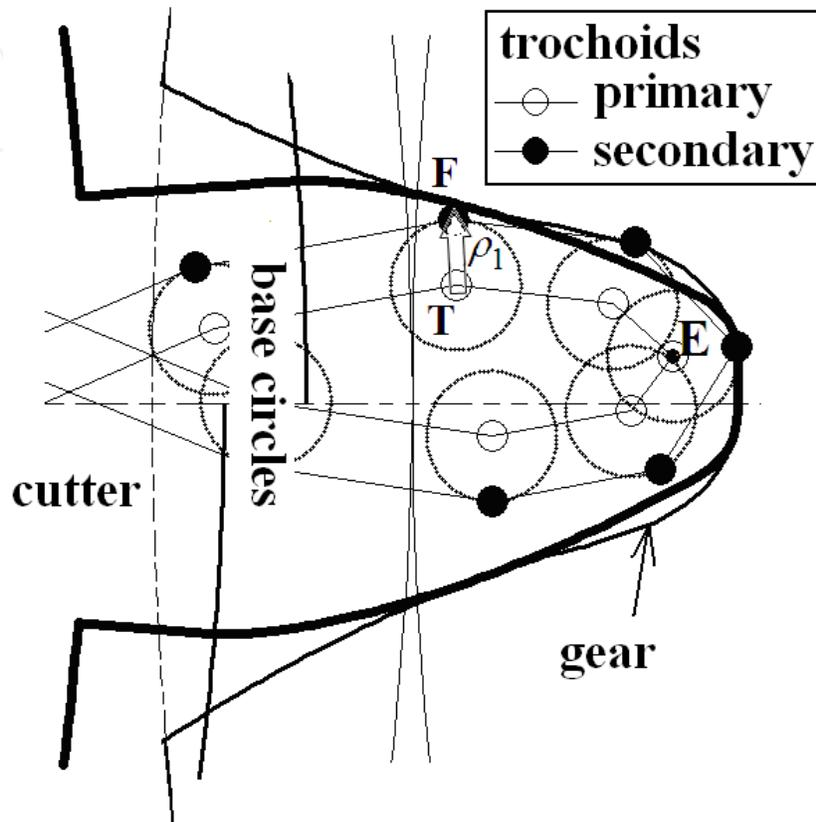
Fig. 7. Trochoidal paths of the pinion-type cutter tip
