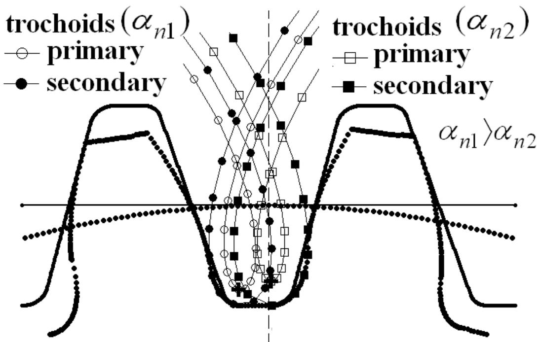
Fig. 8. Trochoidal paths of rack cutter of type-1a
