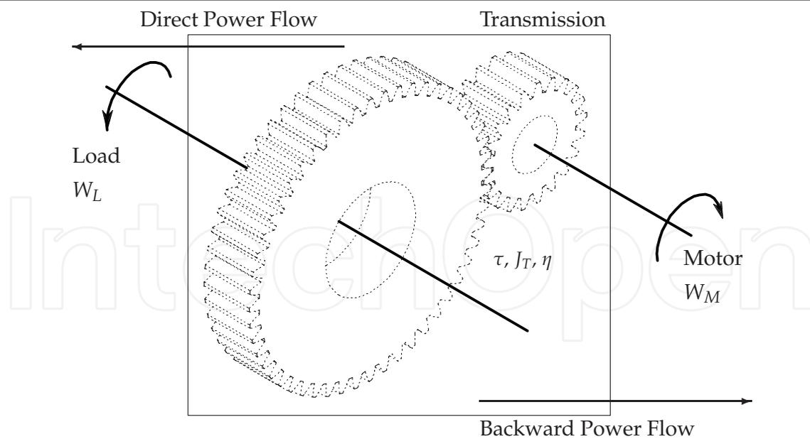
Fig. 1. A scheme of a simple transmission
