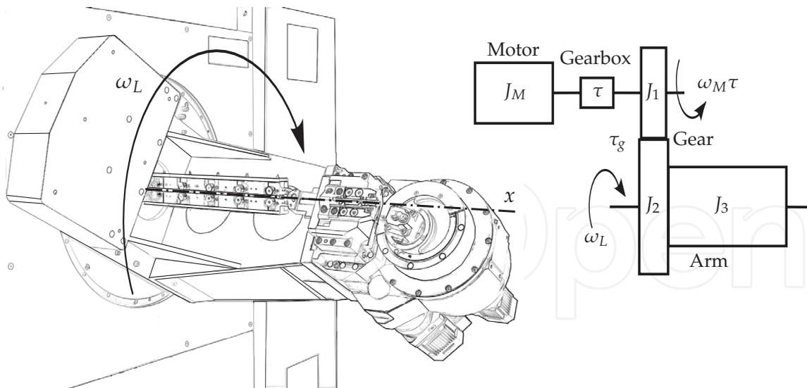
Fig. 6. The moving arm and mechanical system layout
