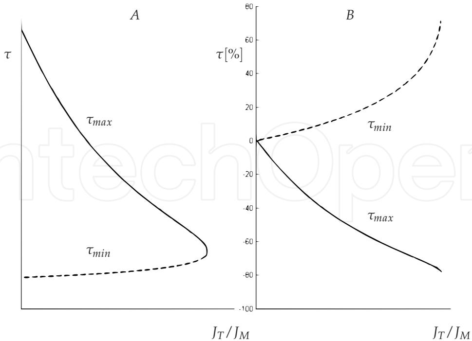
Fig. 12. A - reduction of range of useful transmission ratio as function of  $J_T/J_M$  (for  $T_L = \text{cost}$ ); B - percentage change of maximum and minimum transmission ratios as function of  $J_T/J_M$  (for  $T_L = \text{cost}$ ).
