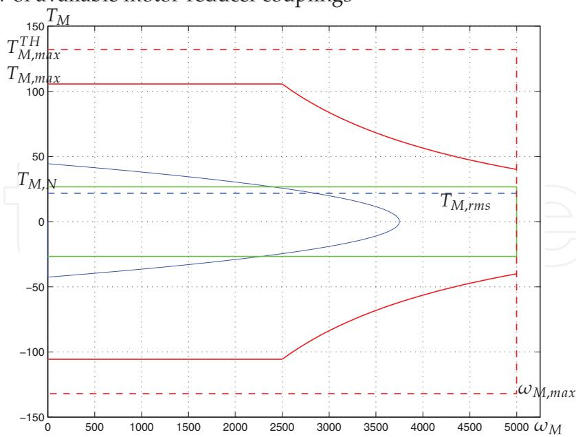
Fig. 9. Checkouts on maximum and nominal torque.
