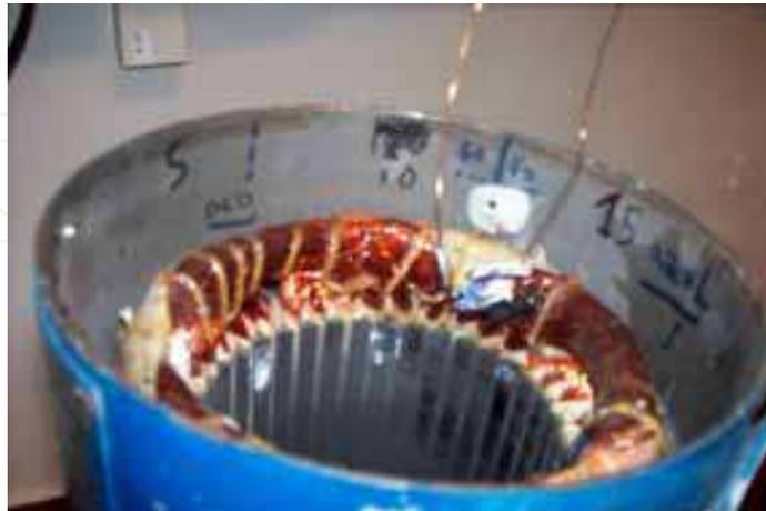
Fig. 8. Induced short-circuit
