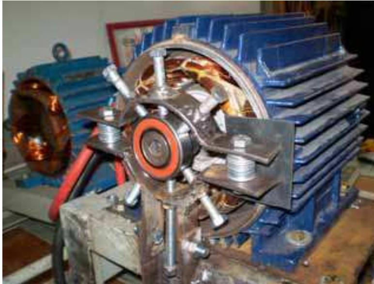
Fig. 14. Eccentricity induced failure
