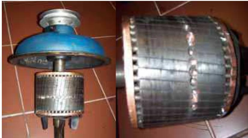
Fig. 3. Rotor perforations
