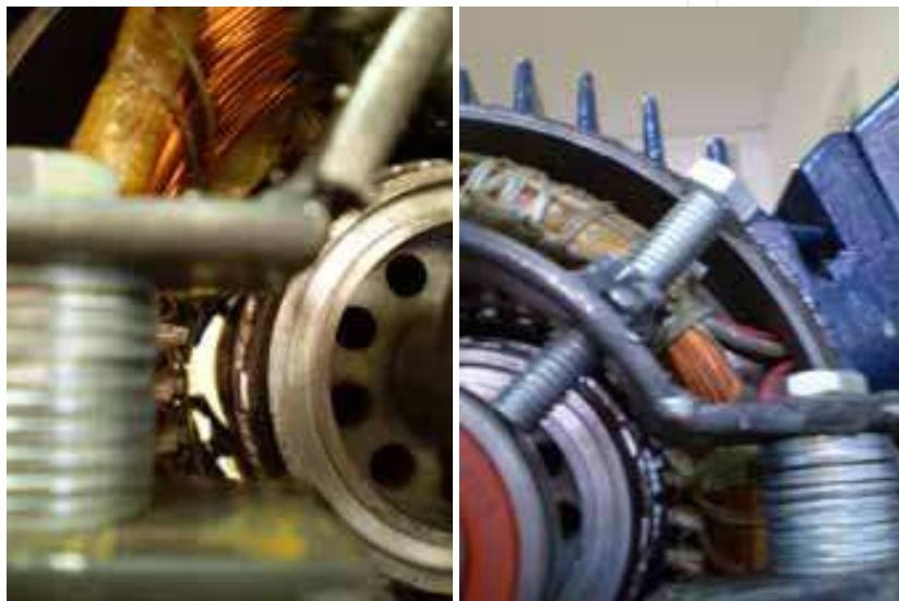
Fig. 18. Eccentricity failure
