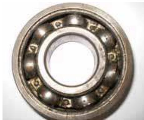
Fig. 13. Bearing damage
