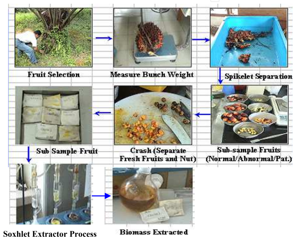
Fig. 3. Bunch Analysis Step Procedure for Oil Extraction
