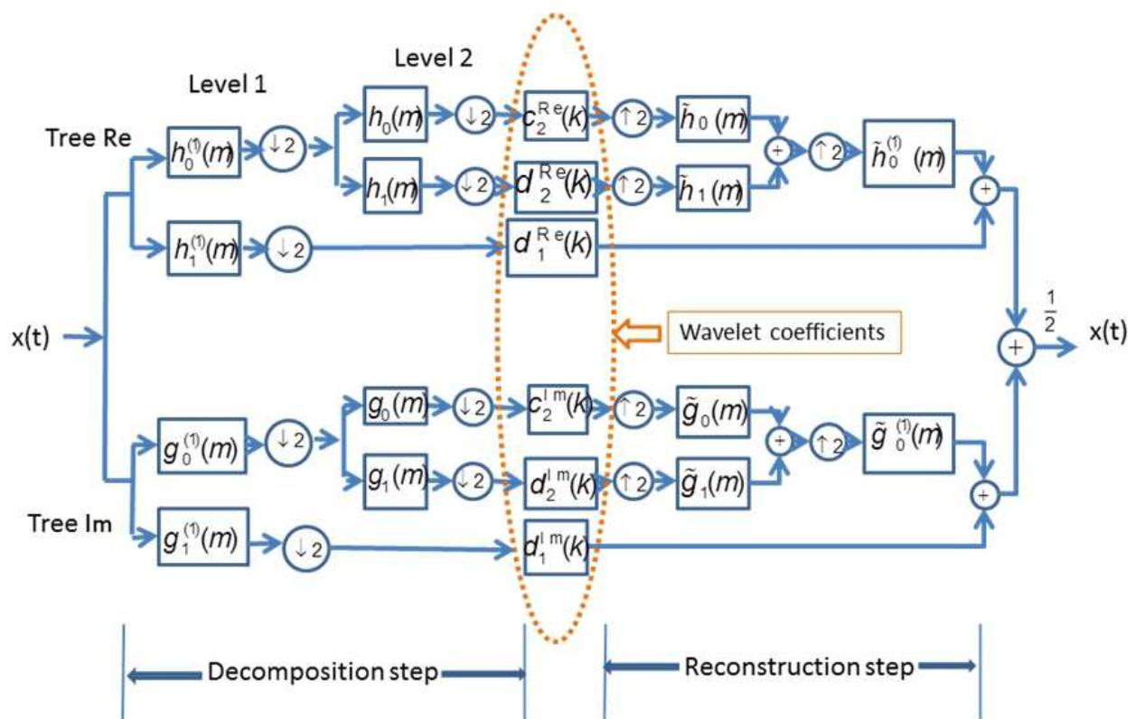
Fig. 3. Decomposition and reconstruction stages of DTCWT
