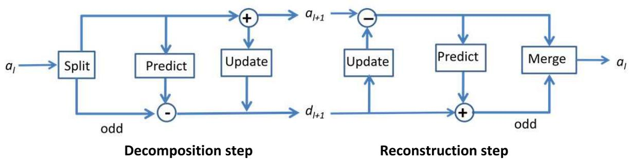
Fig. 6. Decomposition and reconstruction of the signal with SGWT
