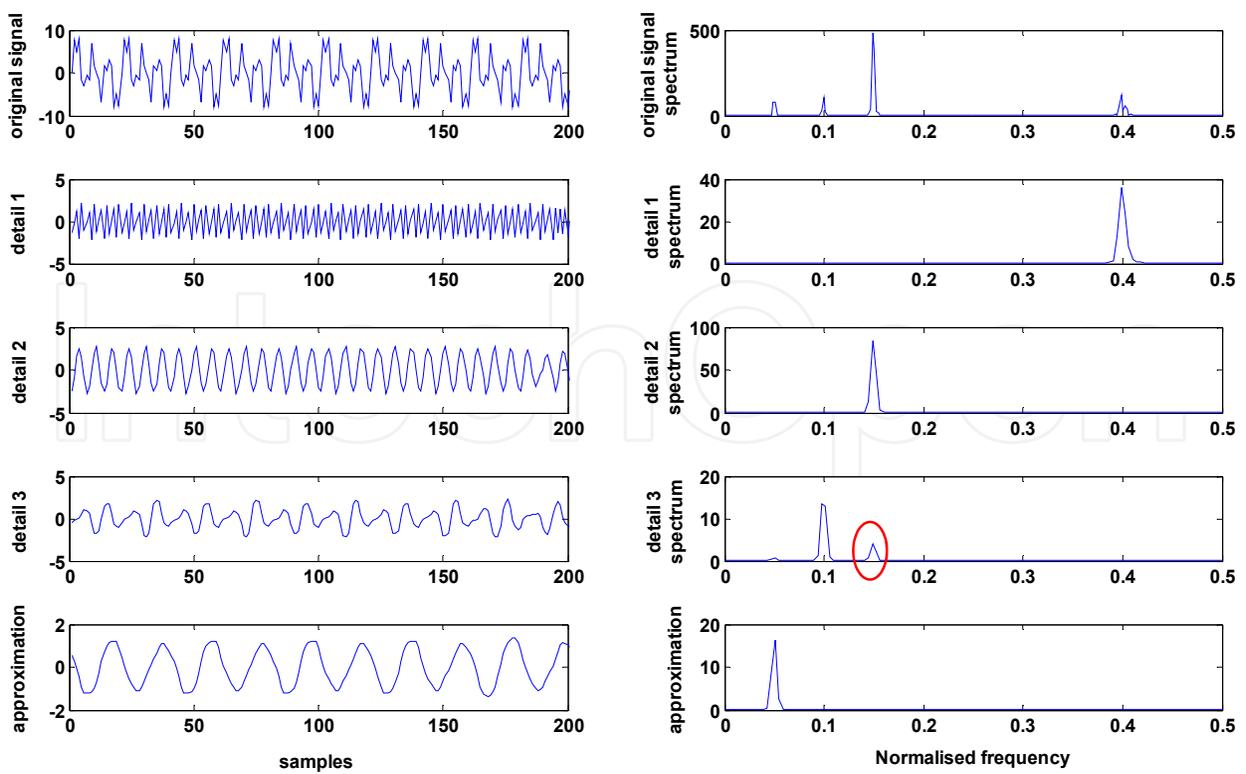
Fig. 5. 3-level decomposition with DTCWT of  $x(t)$
