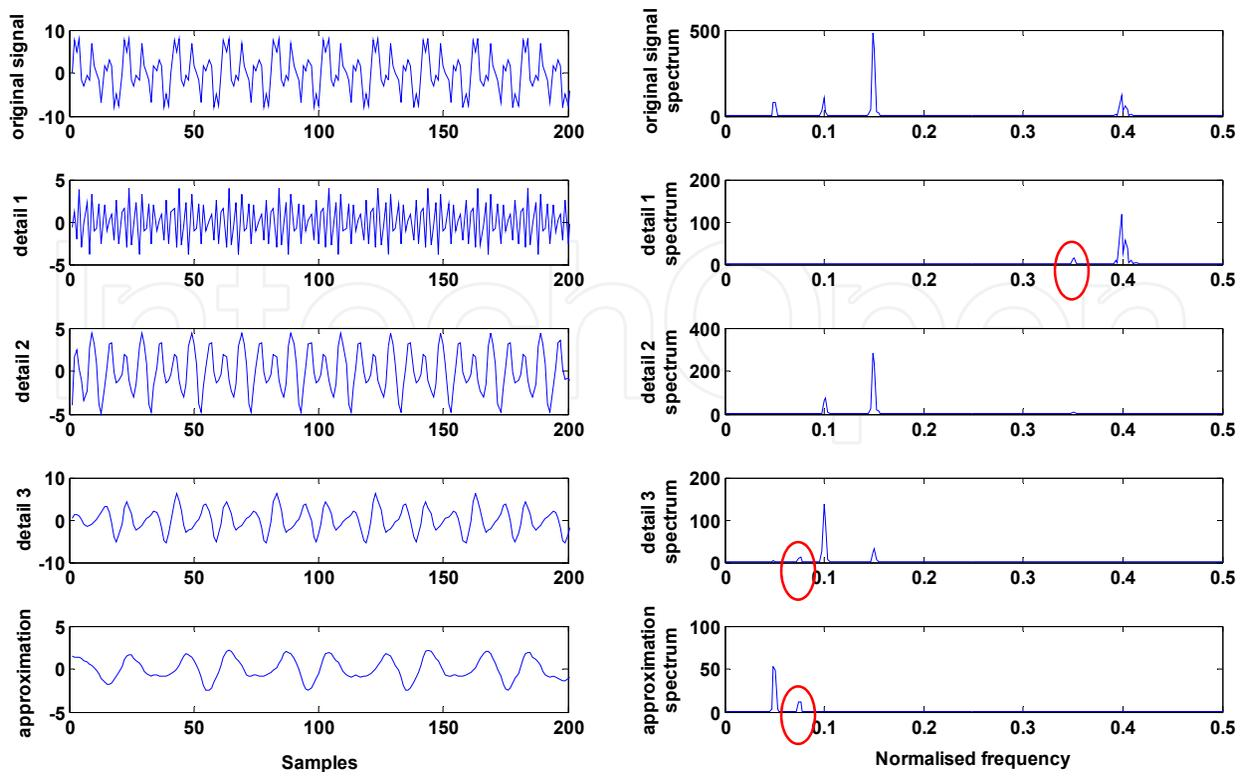
Fig. 4. 3-level decomposition with DWT of  $x(t)$
