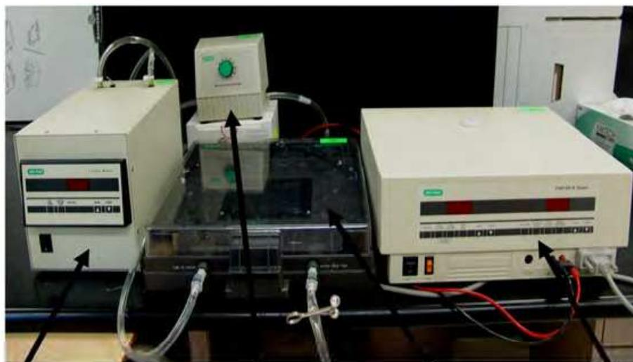
Chiller Pump Electrophoresis chamber Programmed Power Supply
