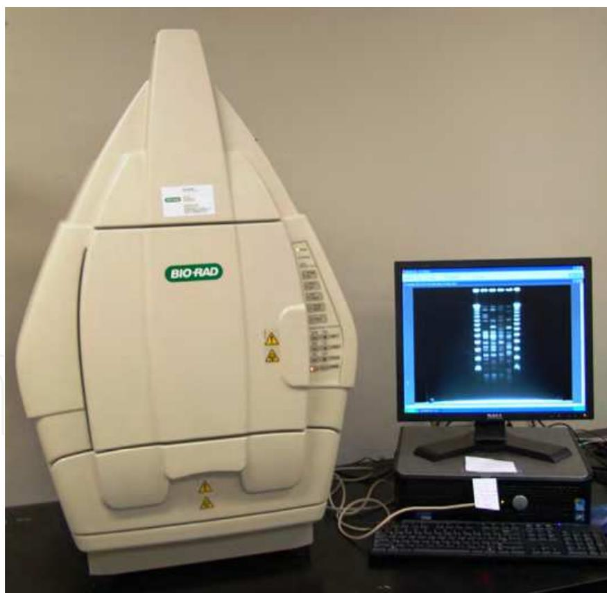
The Gel Doc image system captures picture of the stained gel with the bands and this is transmitted to a computer and monitor for better visualization and analysis
