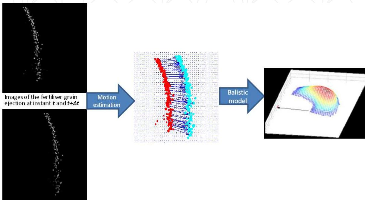
Fig. 3. The images on the left are images of fertilizer grain ejection at the instant  $t$  and  $\Delta t$ ; the middle image shows the displacement vector determined by the motion estimation algorithm, and the right image shows the spread pattern determined from the ballistic model.
