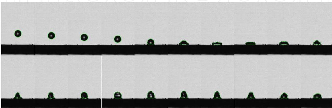
Fig. 6. Sequence of droplet impact with adhesion.
