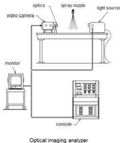
Fig. 1. Typical Particle droplet imaging analyzer (PDIA) (Schick, 1997).
