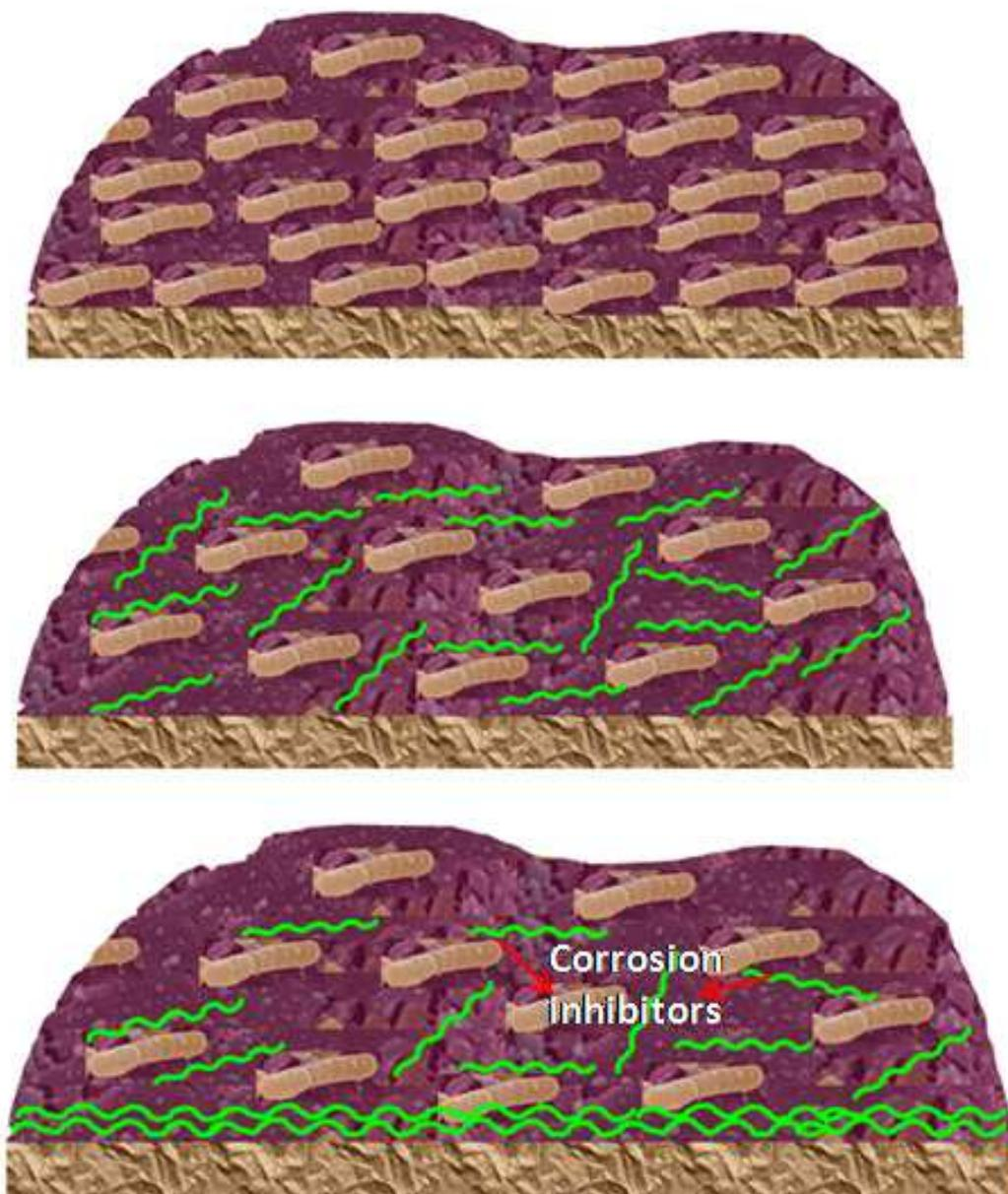
Fig. 9. Corrosion resistance by the formation of biofilm.
