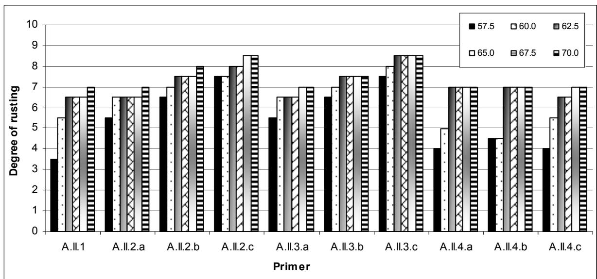
Fig. 4. Coatings based on binder A: Degree of rusting in salt spraying (fog) chamber; average values of failures in X-cut and in general area of panel.
