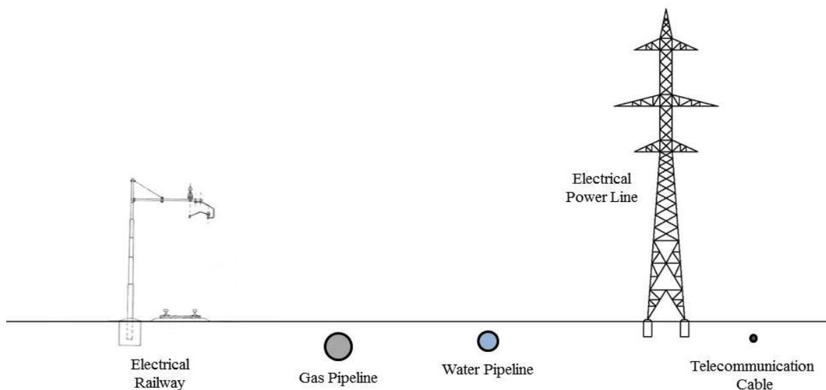
Fig. 1. Common distribution corridor. Right of way.
