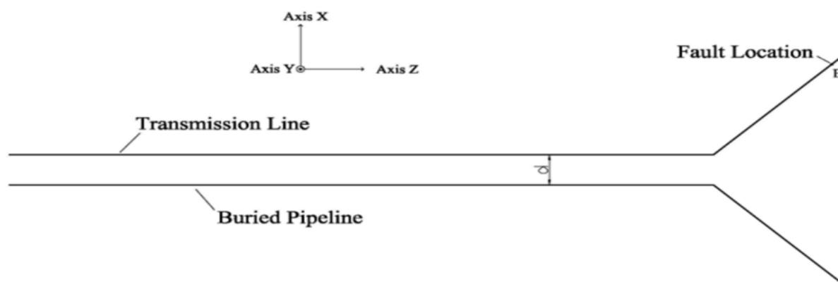
Fig. 3. Top view of the parallel exposure.
