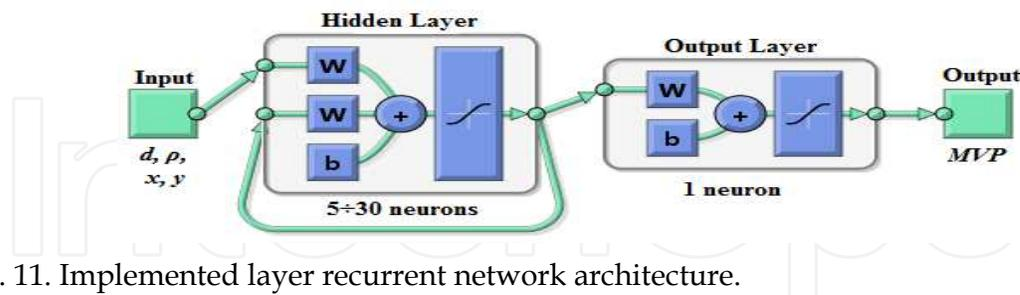
Fig. 11. Implemented layer recurrent network architecture.
