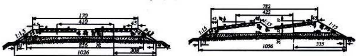
Fig. 5. Sections of railway track in the former Soviet Union (the dimensions are in cm)
