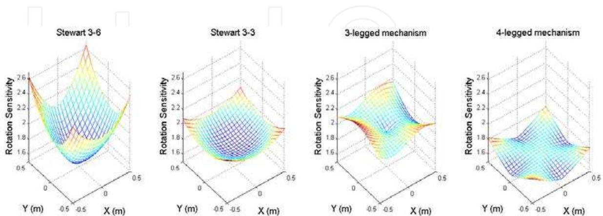
Fig. 10. Rotation Sensitivity index of Stewart 6-6, Stewart 3-6, 3-Legged mechanism and 4-legged mechanism on the plane  $z=0.75$  m.
