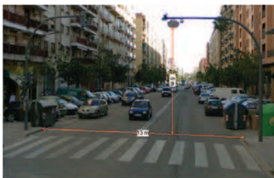
(a) Laser Scanner Positioning
