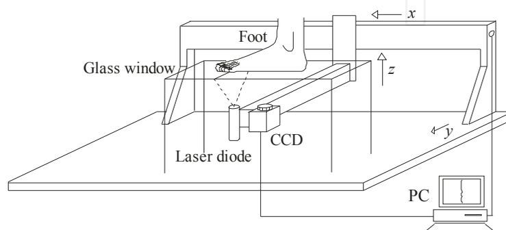
Fig. 1. Experimental setup for foot sole scanning.
