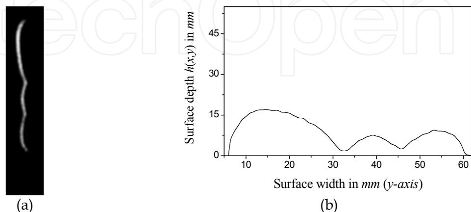
Fig. 3. (a) Laser line projected on the foot sole mould. (b) Surface depth computed by the network form the laser line Fig.3 (a).
