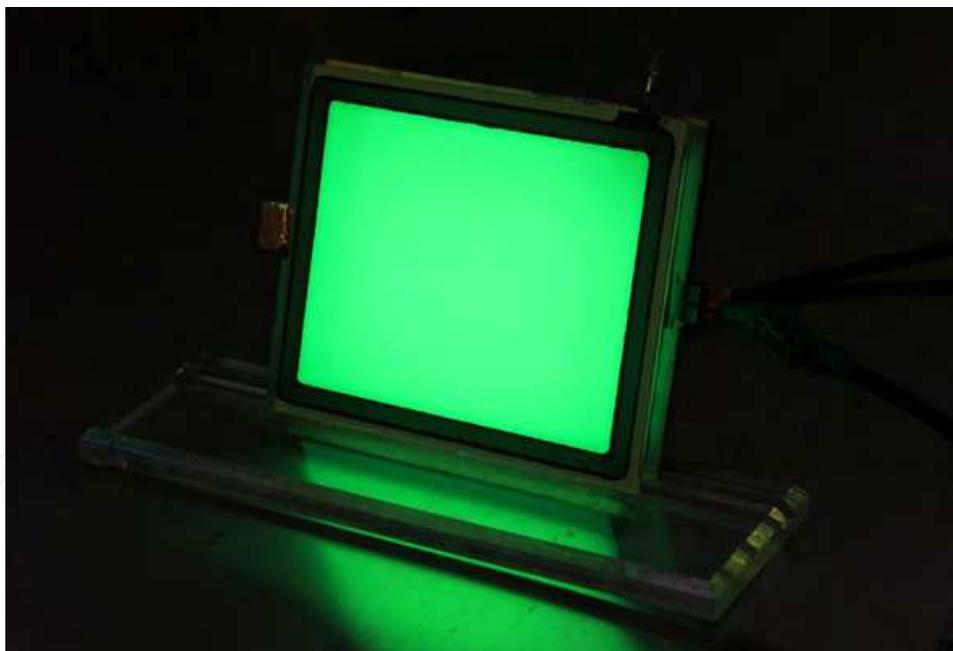
Fig. 2. The photo shows the lighting screen of a typical FEEL device demonstrating the uniform light radiation and absence of dark points ubiquitously encountered in traditional FED devices.
