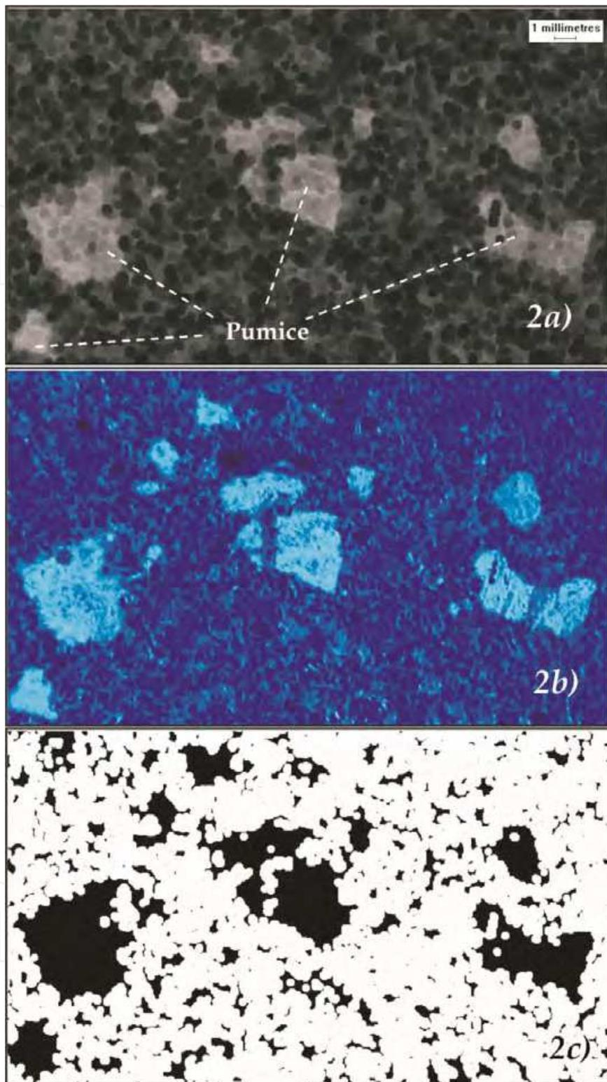
Fig. 4. Photomicrographs of sand-pumice substrate: 2a) greyscale; 2b) ultraviolet light and 2c) binary format. The pumice particles increase the porous space of sand
