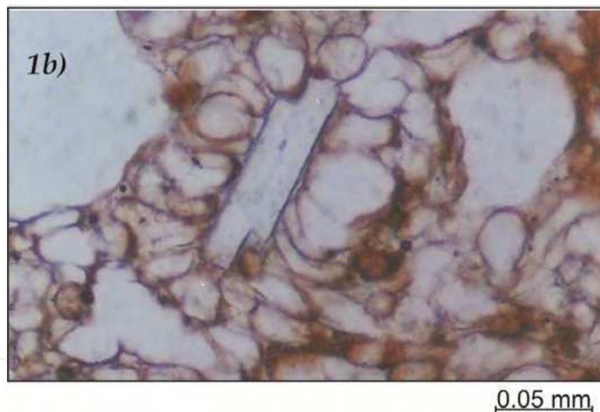
Fig. 3. Photomicrographs of a pumice particle: 1a) pumice particle with incident light, 1b) pumice porous in thin section with plane polarized light
