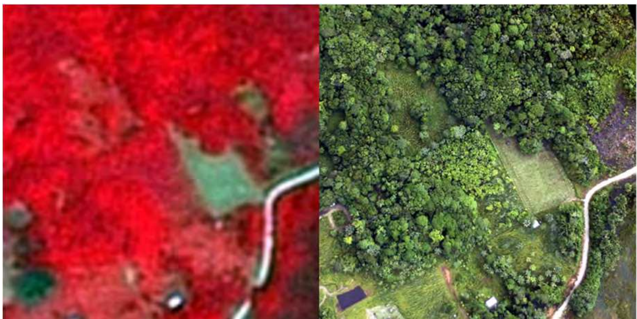
Fig. 1. Differences of canopy grain perception between two 300 m square subset images of different spatial resolution over a mixed savanna forest-inhabited area, French Guiana. Left: a 2.5-m SPOT5 Fusion image acquired in October 2010. Right: a 20-cm aerial photograph acquired in July 2010 (© L'Avion Jaune).
