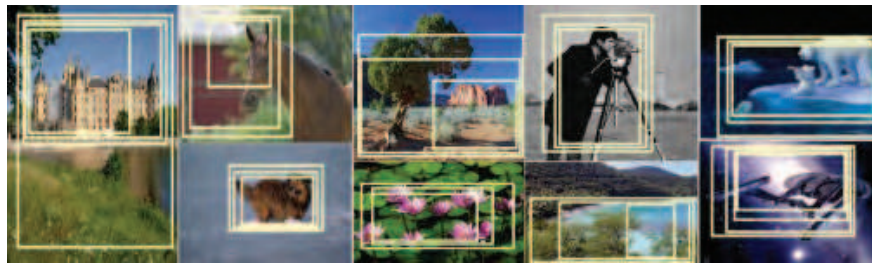
Fig. 14. Example of images along with rectangles providing different attention-based automatic zooms. After a saliency map (Mancas (2009)) is computed and low-pass filtered, several threshold values are used to extract the bounding boxes of the more interesting areas. Depending on this threshold, the zoom is more or less precise/important.
