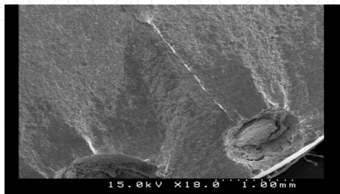
Fig. 4. Fatigue failure arrester at interior pitting deep
