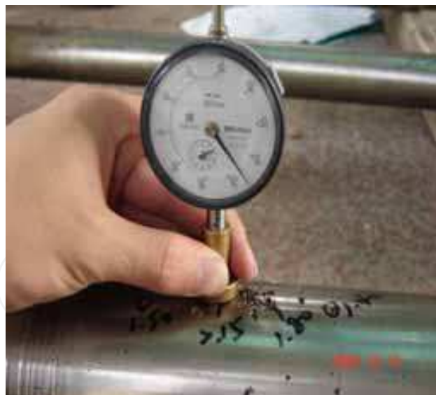
Fig. 2. Measuring depth of pitting deep
