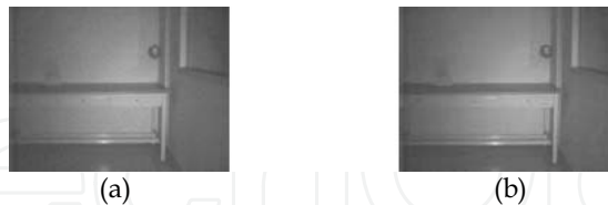
Figure 8. (a) Input low light-level image with significant noise and (b) NAST filtered image Comparison between DoG-based SIFT and the proposed DoW methods is shown in Fig. 9. As shown in Fig. 8, the proposed DoW method outperforms the DoG-based SIFT in the sense of both stability of extracted keypoints and computational efficiency. Fig. 10, Compares performance of combined NAST and DoG method with the DoG-based SIFT algorithm.
