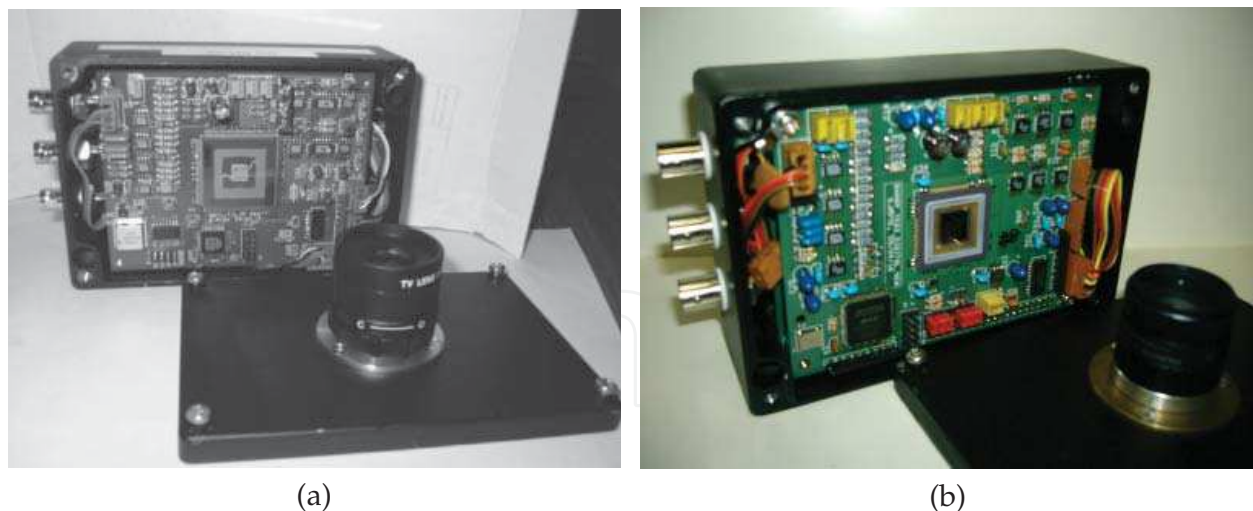
Fig. 2. Photographs of CIS cameras with CMOS chips of (a) 64 \times 64 -pixel and (b) 200 \times 200 -pixel sensors.
