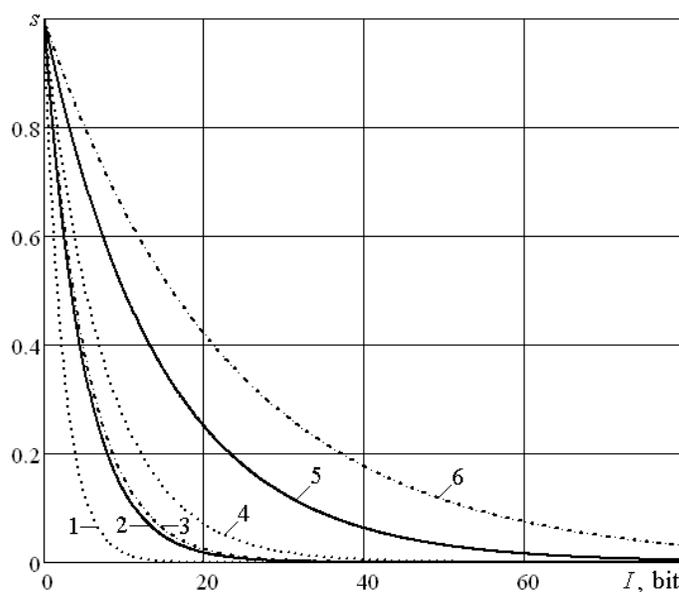
Fig. 2. Composite probability of attack non-detection  $s$  for the ping-pong protocol with many-qubit GHZ-states:  $n=2$ , original protocol (1);  $n=2$ , with superdense coding (2);  $n=3$  (3);  $n=5$  (4);  $n=10$  (5);  $n=16$  (6).  $I$  is Eve's information.
