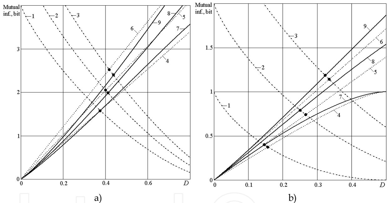
Fig. 1. Mutual information for non-coherent attack. 1, 2, 3 –  $I_{AB}(D)$  for  $d = 2, 4, 8$  (a) and  $d = 16, 32, 64$  (b); 4, 5, 6 –  $I_{AE}^{(d+1)}(D)$  for  $d = 2, 4, 8$  (a) and  $d = 16, 32, 64$  (b); 7, 8, 9 –  $I_{AE}^{(2)}(D)$  for  $d = 2, 4, 8$  (a) and  $d = 16, 32, 64$  (b).
