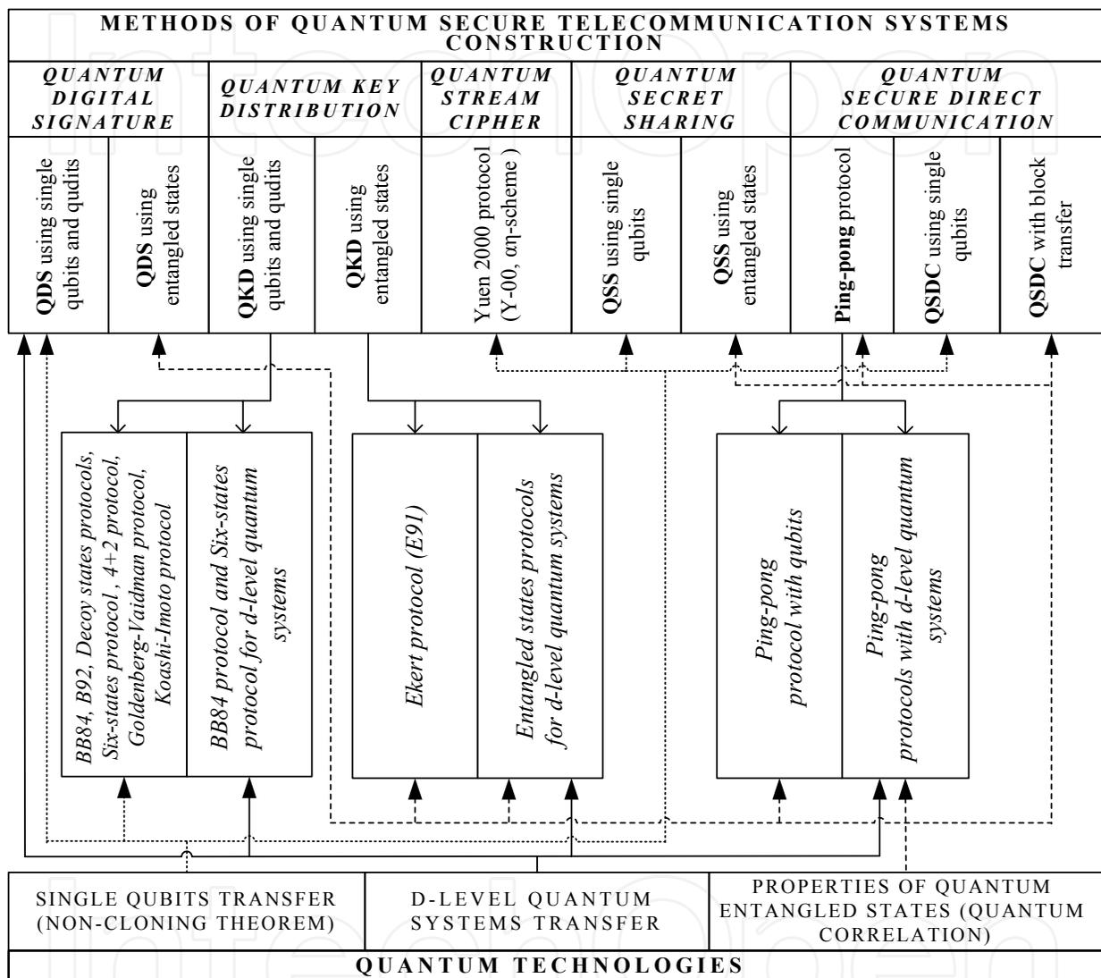
Fig. 4. Methods of quantum secure telecommunication systems construction.
