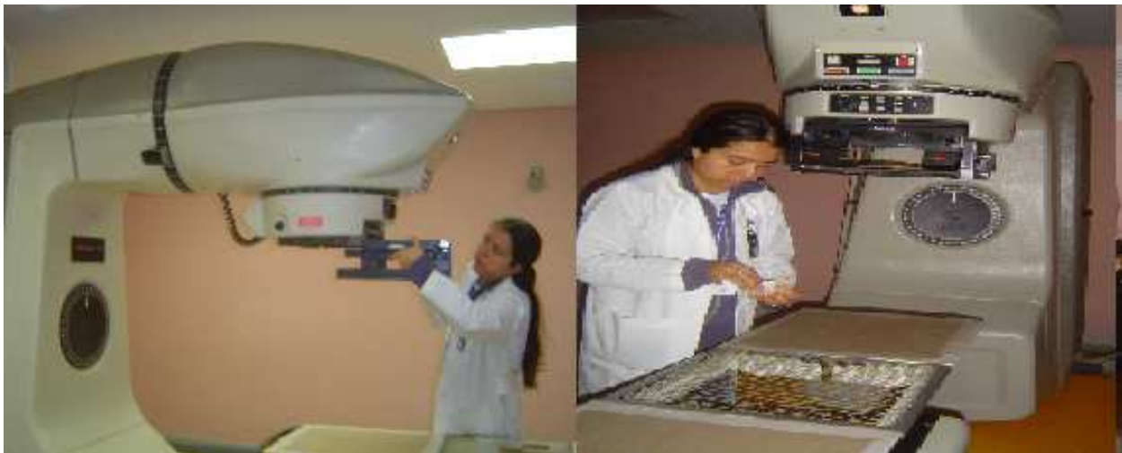
Fig. 1. Cobalt 60 Unit (Theraton 780e), used for irradiation of seeds of Abies religiosa and Pinus hartwegii , located in Centro Estatal de Cancerología de Xalapa, Veracruz, Mex.
