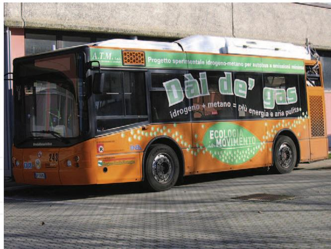
Fig. 15. Urban bus tested with HCNG blends (Genovese et al., 2011).
