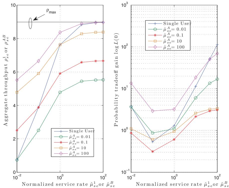
Fig. 11. Comparison of single and two SU groups, **Left:** Aggregate Throughput, and **Right:** tradeoff gain versus normalized SU service rate given  $\theta_p = 1, \theta_{se}^1 = 12, \theta_{se}^A = 6, \theta_{se}^B = 6$  and  $r = 0$ .
