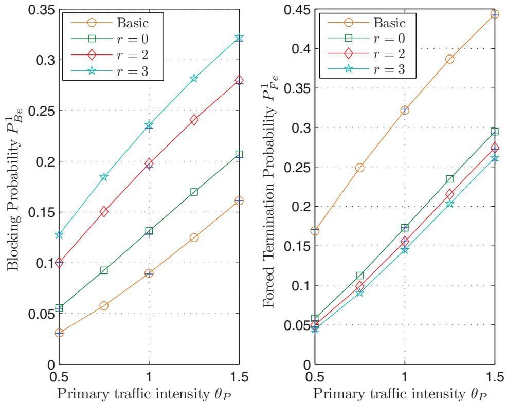
Fig. 8. Single SU group, **Left:** Blocking probability, and **Right:** Forced termination probability versus PU traffic intensity given  $\theta_{se}^1 = 8$  and  $\hat{\mu}_{se}^1 = 1$ . Simulation results are shown with “+”.
