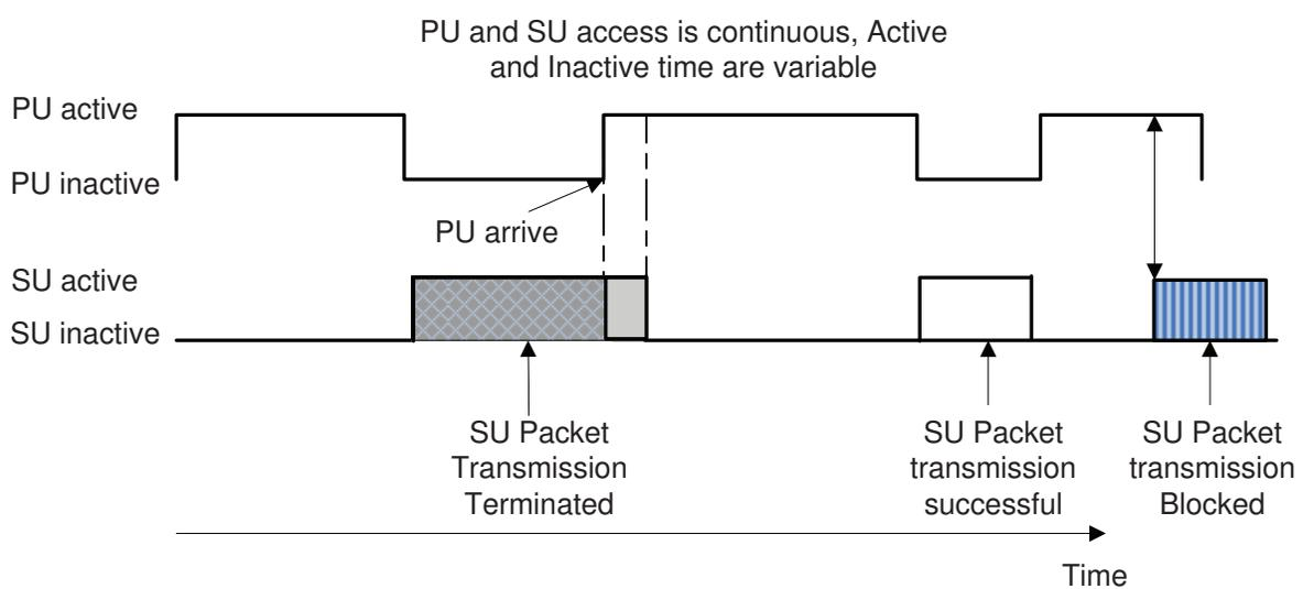
Fig. 2. Illustration of forced termination and blocking
