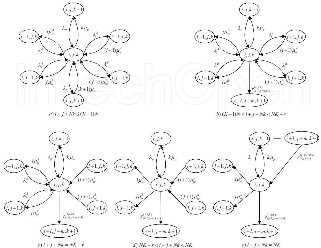
Fig. 7. A CTMC for the system with spectrum handoff and channel reservation  $r < N$ . The states  $(i - l, j - m, k + 1)$  satisfy packing condition i.e.,  $(i - l) + (j - m) = (K - k - 1)N$  for  $0 < l + m \leq N$ .
