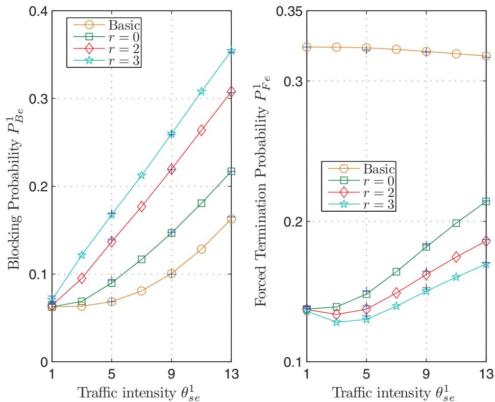
Fig. 9. Single SU group, **Left:** Blocking probability, and **Right:** Forced termination probability versus SU traffic intensity given  $\theta_p = 1$  and  $\hat{\mu}_{se}^1 = 1$ . Simulation results are shown with “+”.
