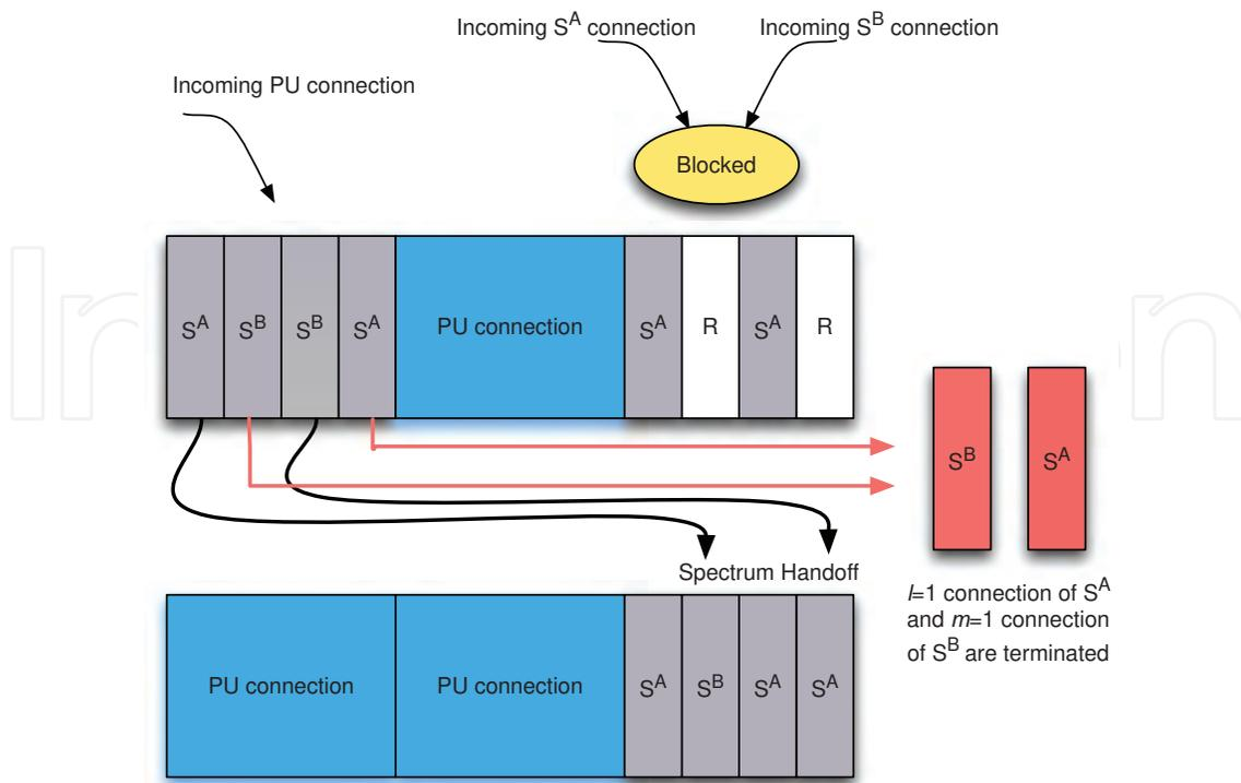
Fig. 6. Illustration of the system with spectrum handoff and channel reservation. The number of reserved channels  $r = 2$ .
