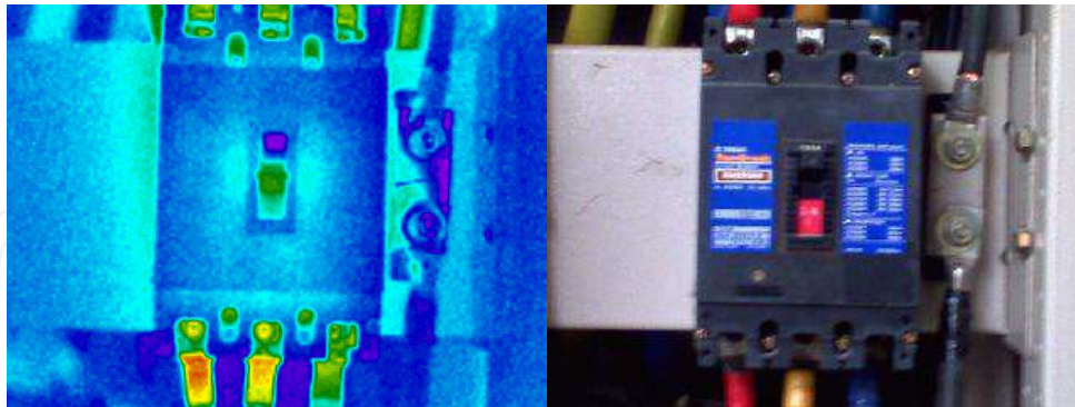
Fig. 3. Infrared image and visible light image
