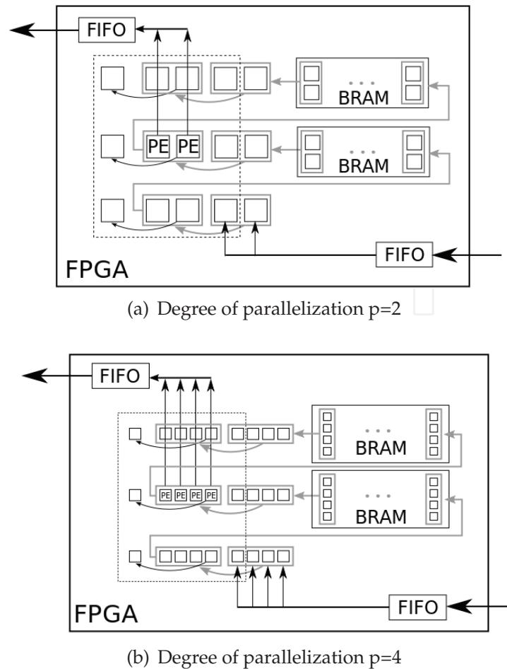
Fig. 6. Generic Full Buffering template for streaming applications
