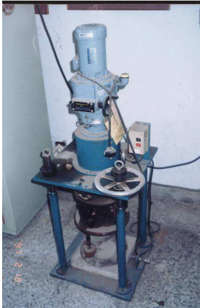
Fig. 2.3. Revolving disk abrasion test machine
