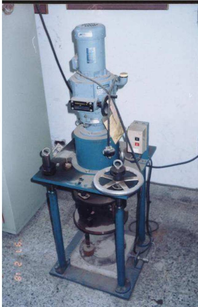
Fig. 2.3. Revolving disk abrasion test machine
